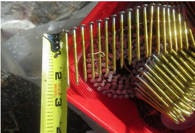
8d nails used on all Tamarind roof decks
